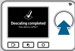
As soon as “Descaling completed” is displayed, the descaling process is finished. The red maintenance menu button
